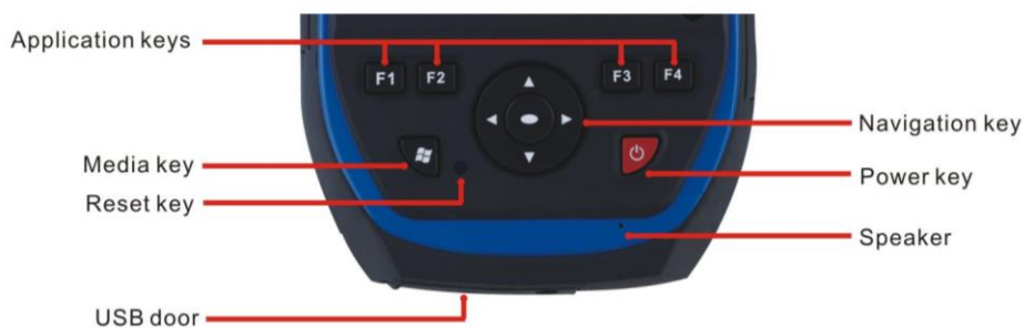
Figure 2.1.2 - S7G handheld keypad area
